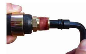
5. Insert lock stem. Then turn and push with the wrench until flush with the fitting.
