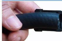
1. Cut off damaged end of hose. Position hose end on the inside groove of the plastic case.
